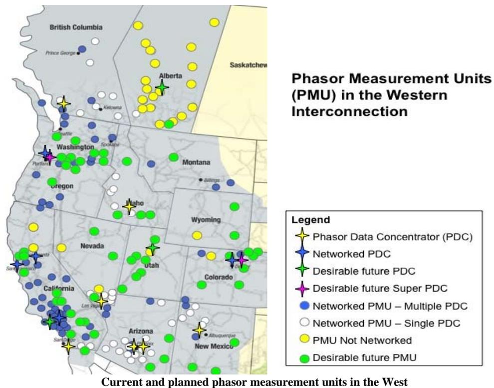
These improvements together will make the power system more reliable. BPA Technology Innovation Office is currently funding several projects that are directly linked to WISP objectives. Inter-area Oscillation Damping project looks at the ways to use wide-area synchro-phasor data to detect large unstable oscillations before they become a problem. Real-time monitoring gives operators the situational awareness information needed for smart decision making and control. Voltage Stability Control
