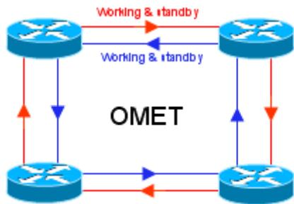
**4 PMU substation network ring**
