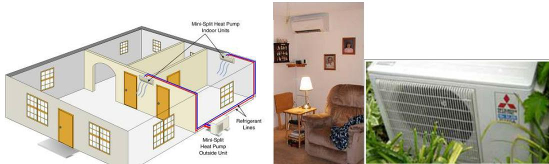
**Home Schematic Layout Drawing and Pictures of Inside and Outside Units**
