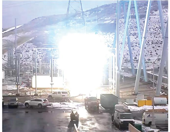
*BPA staged-fault tested at the Celilo Converter Station.*
